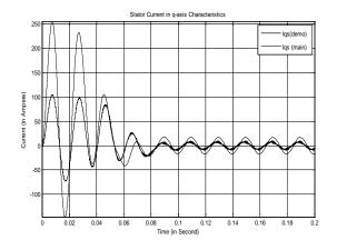
Fig.6.1 Stator Current in q- axis versus time curves (iqs vs. time)
