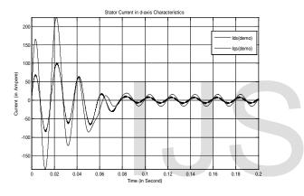
Fig.6.2 Stator Current in d- axis versus time curves (ids vs. time)
