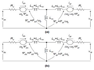
Fig 3.1 d-q equivalent circuit of an Induction Machine
