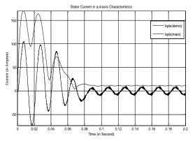
Fig.6.3 Stator Current in dq- axis versus time curves ( $i_{qds}$  VS. time)
