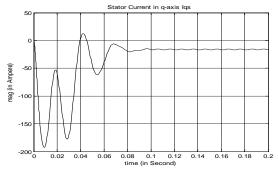
Fig.5.1 Stator Current in q- axis versus time curves (iqs vs. time)
